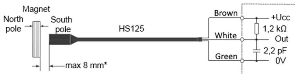
Fig. 2 HS125 connection scheme
